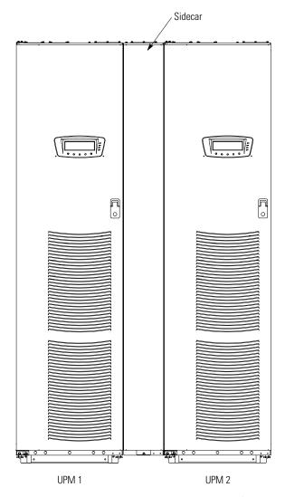
Figure 2-2. Typical Line-up-and-Match Parallel Redundant System (80 kVA System Shown)
